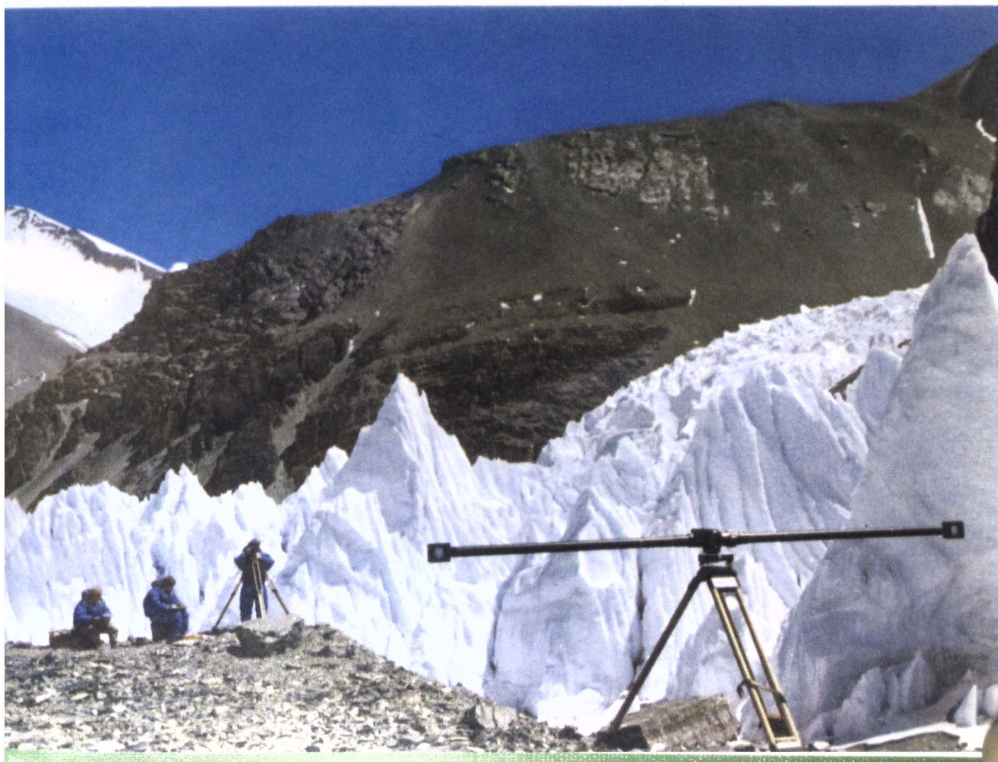
Measuring a base line for terrestrial stereophotogrammetric surveying on medial moraine of East Rongbuk Glacier.
